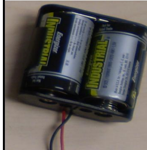
DEXEN BACKUP BATTERY PACK
