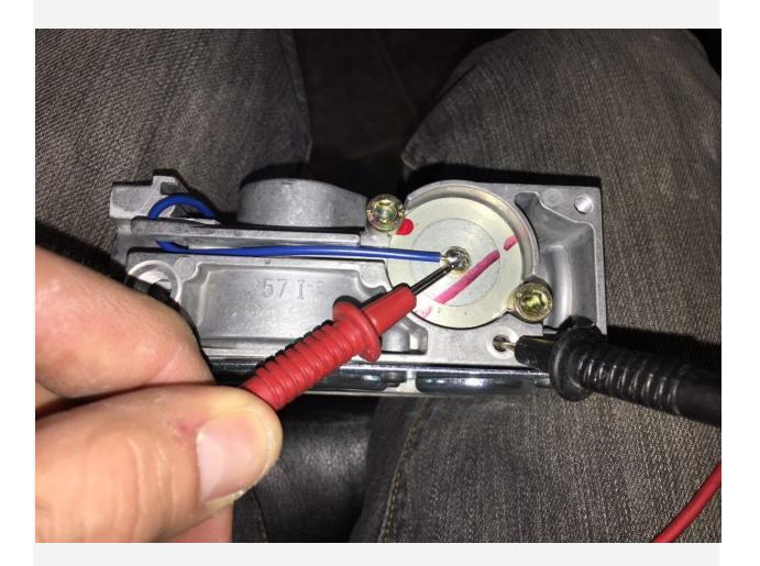
A good reading here is anywhere between 0 and 0.2. If it is more than 0.2 then replace the valve.
